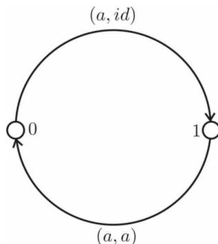
FIGURE 4. Dual Moore diagram of the adding machine
